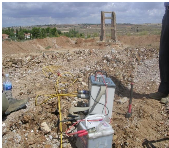
Photo of the electrical scans of the mines
